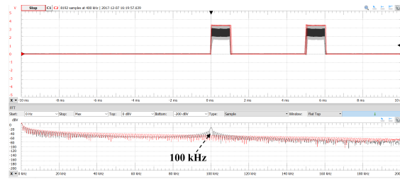
Fig. 8: Transmitted and reproduced signal in time and frequency domain
