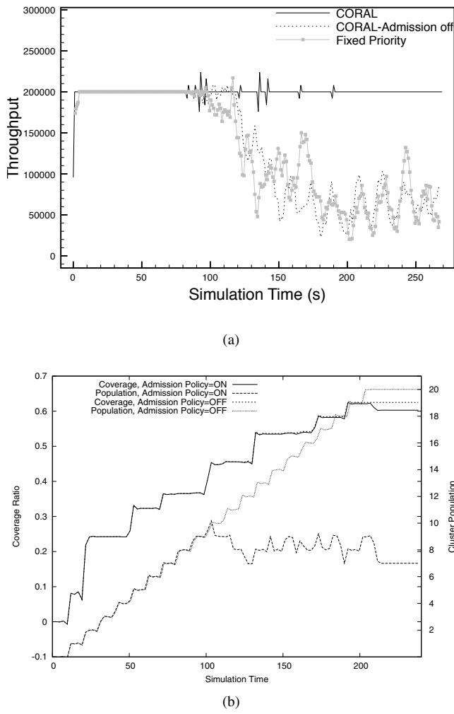
Fig. 3. Meeting bandwidth requests of incoming MCs for 200 Kbps (a), the relationship between coverage ratio and number of MCs in a cluster (b), respectively.
