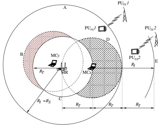
Fig. 1. The transmission and interference ranges in a CR WMN cluster.
