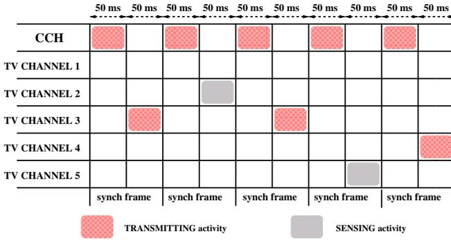
Fig. 2. The channel model for  $M = 5$  and  $T_s=150$ ms.
