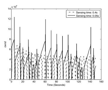
Fig. 8. cwnd of Westwood+ with different sensing times
