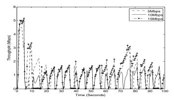
Fig. 4. Real-time throughput of NewReno for different channel bandwidths
