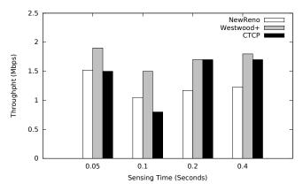
Fig. 7. Average throughput of NewReno, Westwood+, CTCP with different sensing times
