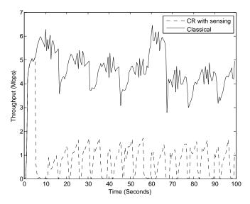
Fig. 2. Real-time throughput of NewReno in cognitive radio network and none-cognitive radio network
