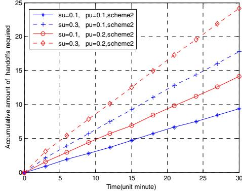
Figure 7. The accumulative amount of handoffs required by SUs in scheme 2 when both  $\lambda_{PU}$  and  $\lambda_{SU}$  change
