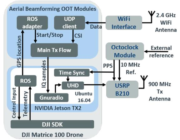
Fig. 8: UAS solution stack consisting both hardware and software components.
