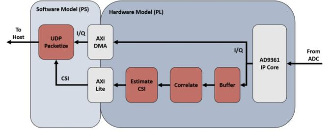
Fig. 12: A high level block diagram of the hardware and software processing blocks for the beamforming receiver
