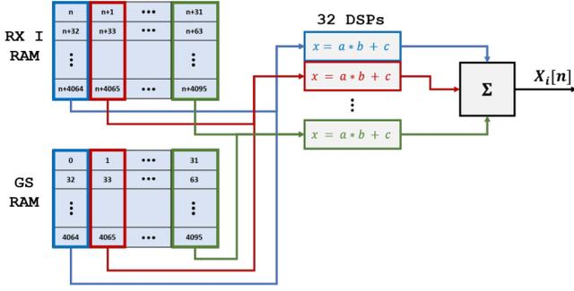
Fig. 13: A block diagram showing the correlation computation for a single sample  $X_i[n]$  or  $X_q[n]$ .
