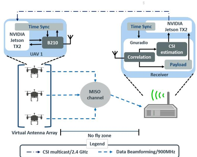
Fig. 1: System architecture for AirBeam
