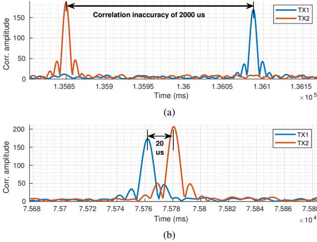
Fig. 9: Timing synchronization issues before (a) and after (b) moving to our proposed hardware based approach.
