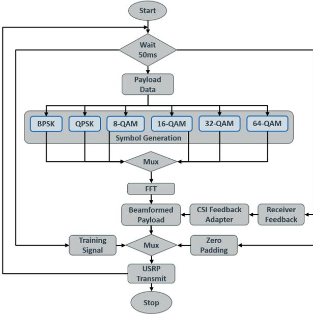
Fig. 7: GnuRadio based Aerial Transmit Beamforming Algorithm.
