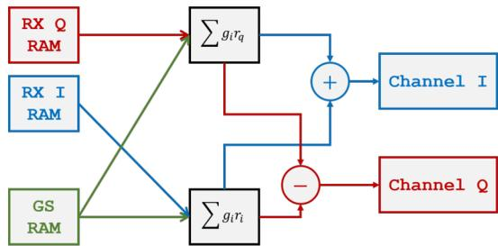
Fig. 14: A block diagram showing the least-squares computation for CSI estimation.
