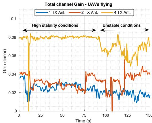
Fig. 16: Channel gain ( $|\mathbf{h}^H \mathbf{h}|$ ) with 1, 2 and 4 antennas.
