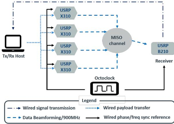
Fig. 3: Architecture of static on-ground test-bed setup evaluating multi-user transmit beamforming.
