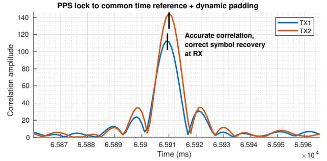
Fig. 10: Accurate cross-correlation within 1  $\mu$ s accuracy with time sync and delay mechanism enabled.
