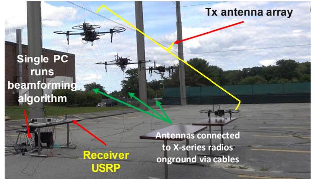
Fig. 5: UAS test-bed setup to evaluate multi-user transmit beamforming.
