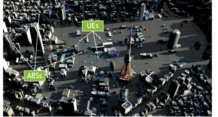
Fig. 8: Live capture of ABS configuration imported from Sionna to AODT. UEs placed in AOI 1 and rays shown for all ABSs and a sample UE.
