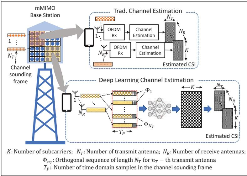
FIGURE 1. Overview of deep-learning-based channel estimation for B5G massive MIMO.
