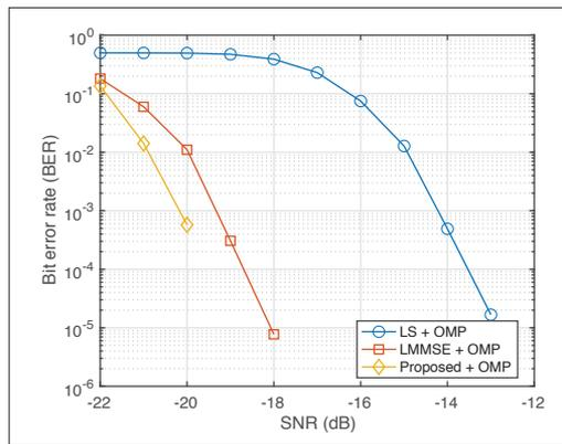
FIGURE 5. BER measured over different SNR level for LS estimation and proposed DNN-based method. Value not showed results in BER = 0.
