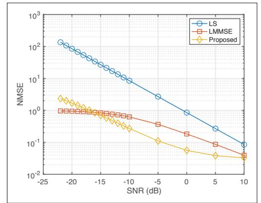
**FIGURE 3.** NMSE between each channel estimation method and ideal channel estimation. Note that as noise power increases, LMMSE output coefficients are close to 0 due to a large amount of noise corrupting the samples, so NMSE approaches 1 as SNR tends to  $-\infty$ .
