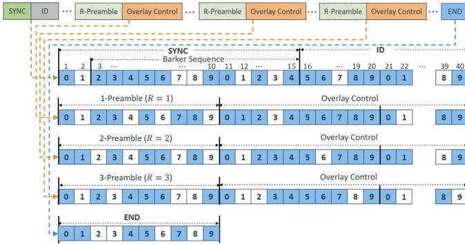
Figure 5: Session management using control signals SYNC, ID, R-Preamble, Overlay Control and End.
