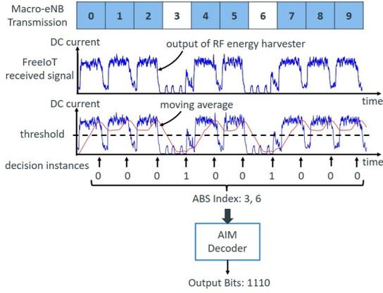
Figure 7: An example of detecting the presence or absence of ABS using the output of RF-EH.
