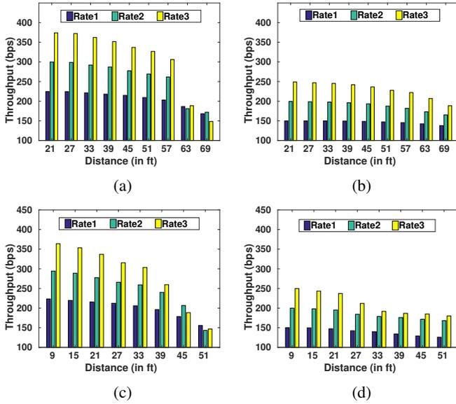
Figure 13: Throughput for baseline *outdoor* receiver scenario (a), and with additional ABS-Code error correction (b). Throughput for *indoor* receiver scenario (c), and with additional ABS-Code error correction (d).
