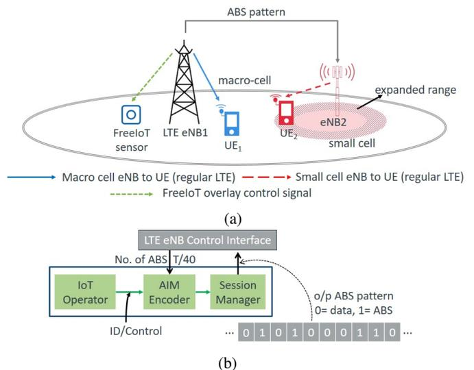
Figure 1: (a) LTE network with the eNB and a given small cell, with spectrum sharing through ABS subframes, (b) FreeIoT framework: The control/wake-up information is conveyed by the position of ABS within a standard LTE frame.
