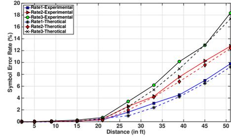
Figure 12: The comparison of the experimental and theoretical SER for the outdoor scenario.
