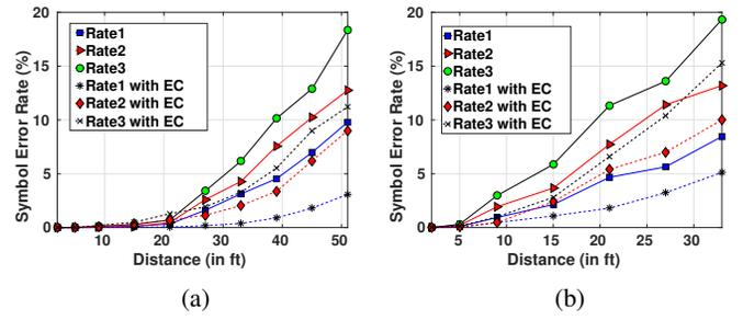
Figure 11: a) The SER for *outdoor* receiver scenario, and b) The SER for *indoor* receiver scenario.
