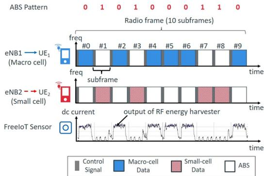
Figure 2: Use of ABS to serve cell edge users of the small cell. FreeIoT sensors detect the ABS pattern using an RF energy harvester.
