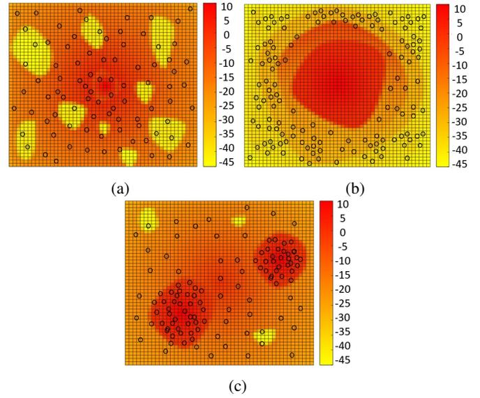
Figure 14: The heatmap of IoT sensors' received power distribution in an area of  $250 \times 250 m^2$  in (a) residential, and (b) stadium, and (c) city downtown.
