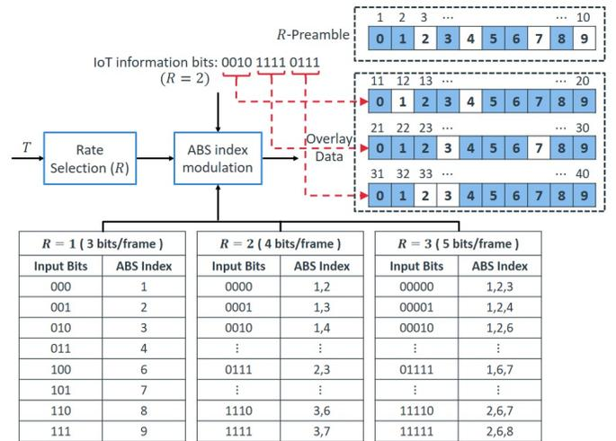
Figure 4: Illustrating rate adaptive ABS Index Modulation. For e.g., for  $R = 2$ , information bits ‘0010’ map to ABS index of ‘1’ and ‘4’ within LTE frame.
