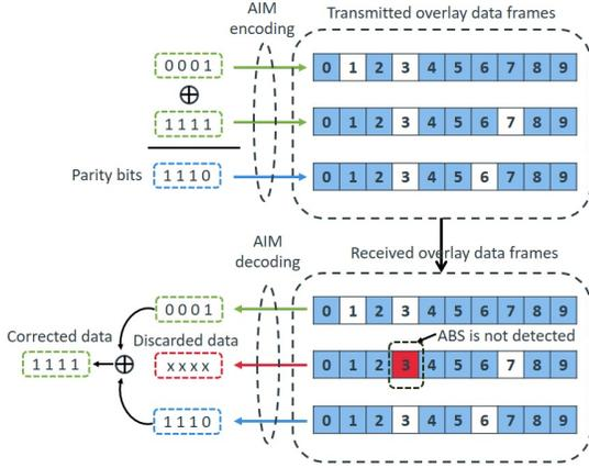
Figure 8: Illustration of ABS-code correction mechanism for rate  $R = 2$ .
