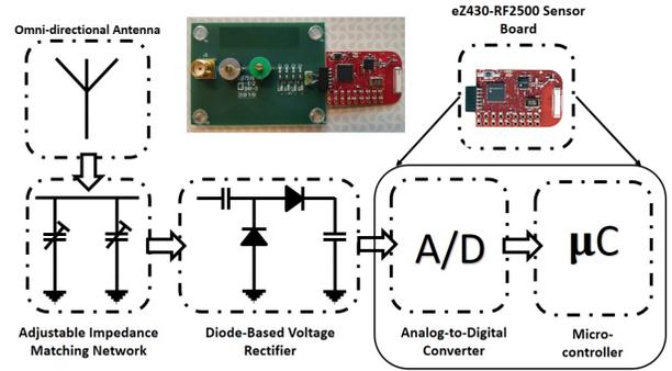
Figure 6: The circuit schematic of FreeIoT receiver.
