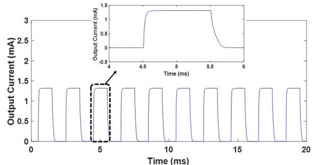
Figure 3: The output current of RF-EH with RF input signal transmitted using OOK modulation with period 1 ms.
