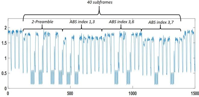
Figure 10: Raw samples of output current of the RF energy harvester for Rate  $R = 2$ . The plots show the ABS pattern of 2 – preamble and overlay control frames with 2 ABS.
