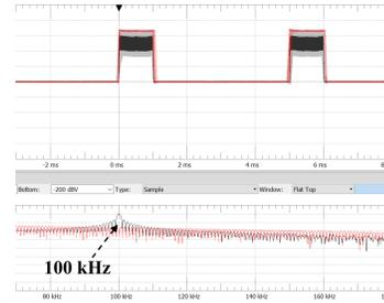
Fig. 8: Transmitted and reproduced signal in time and frequency domain
