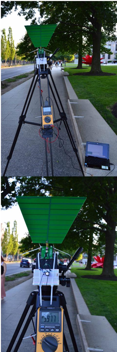
Fig. 24: Battery-free communications setup for performance evaluation at outdoor environment.
