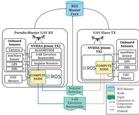
**Figure 4: ROS framework: computational, communication and control elements. ROS runs on a NVIDIA JETSON TX2 mounted on the UAVs. It issues directives to the UAV flight control using IMU and GPS data.**
