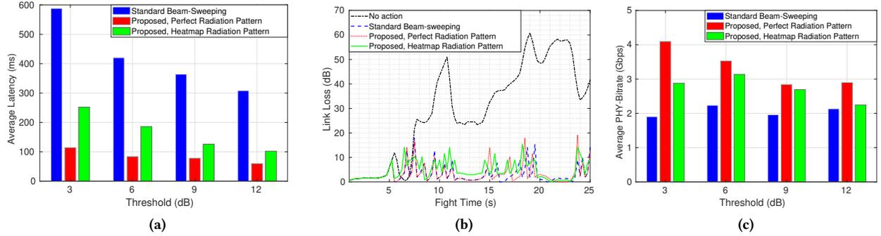
**Figure 5: (a) Average latency in resuming beam-alignment per 1s of emulation time, (b) link loss during emulated flight, threshold for triggering link recovery set to 6 dB (c) average PHY-bitrate including the effect of latency.**
