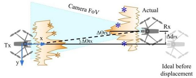
**Figure 1: Beam misalignment caused by UAV translational displacements during hovering. The camera at the Rx helps to coarsely estimate the relative UAV locations, while the beam-patterns are used for fine tuning the correctional movement.**
