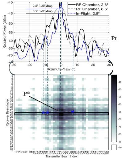
**Figure 2: Extraction of a 2.8° beam pattern from an measured heatmap and comparison with 2.8° and 8.5° beam patterns measured on an RF anechoic chamber.**
