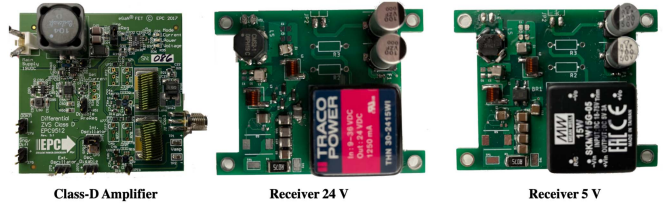
Fig. 6. Class-D amplifier and receiver with different output voltages.
