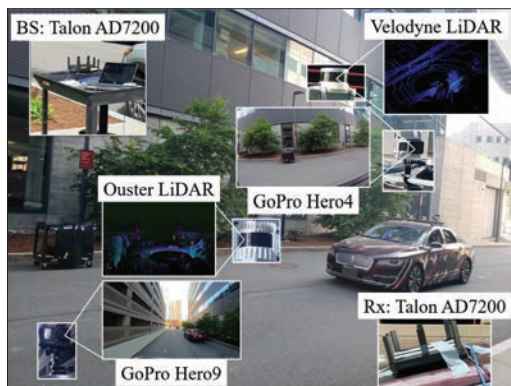
FIGURE 2. The experimental setup of e-FLASH data collection.
