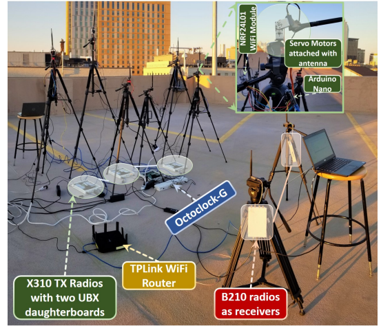
Fig. 7: NetBeam outdoor testbed with a given antenna-location configuration
