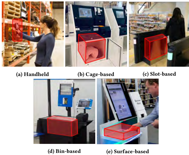
Figure 2: Current RFID-based Self-checkout Systems
