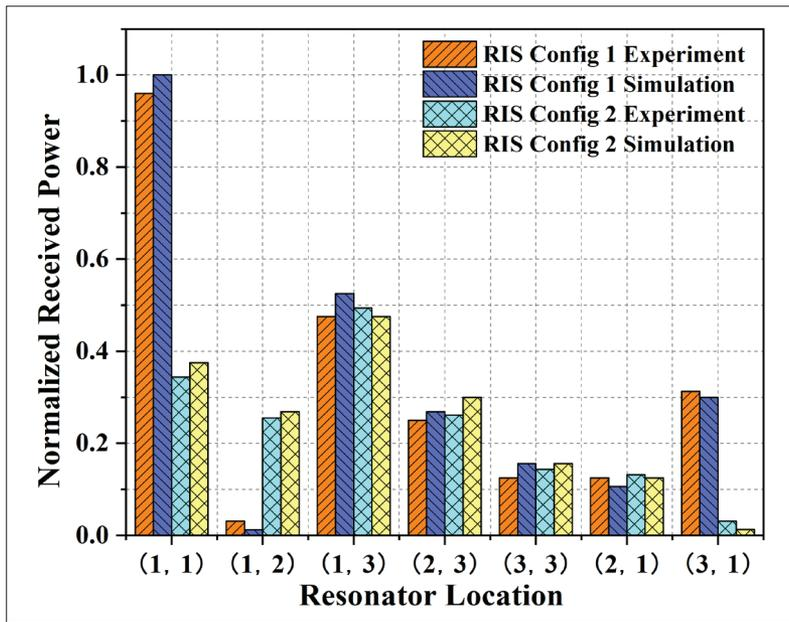
FIGURE 5. Experimental and simulation results of the normalized received power over the 2D surface for different RIS configurations.
