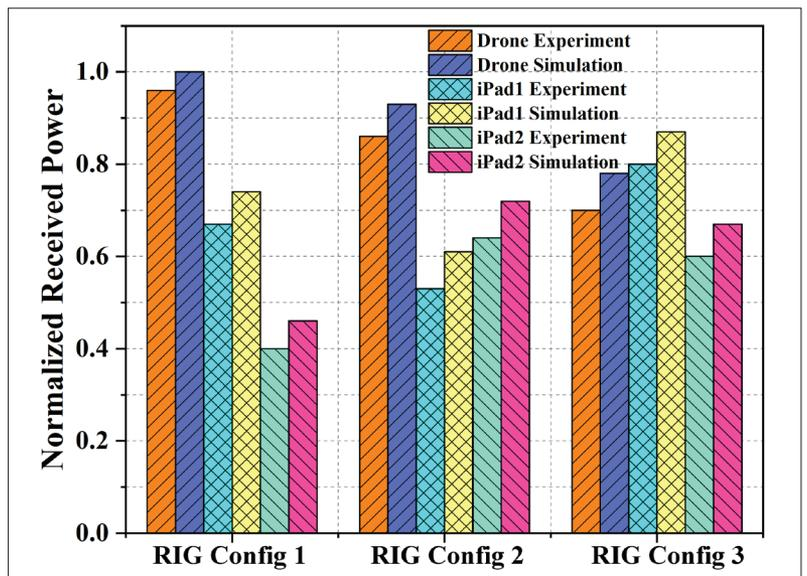
FIGURE 6. Experimental and simulation results of the normalized received power over the 3D surface for iPad and drone over three different RIS configurations.
