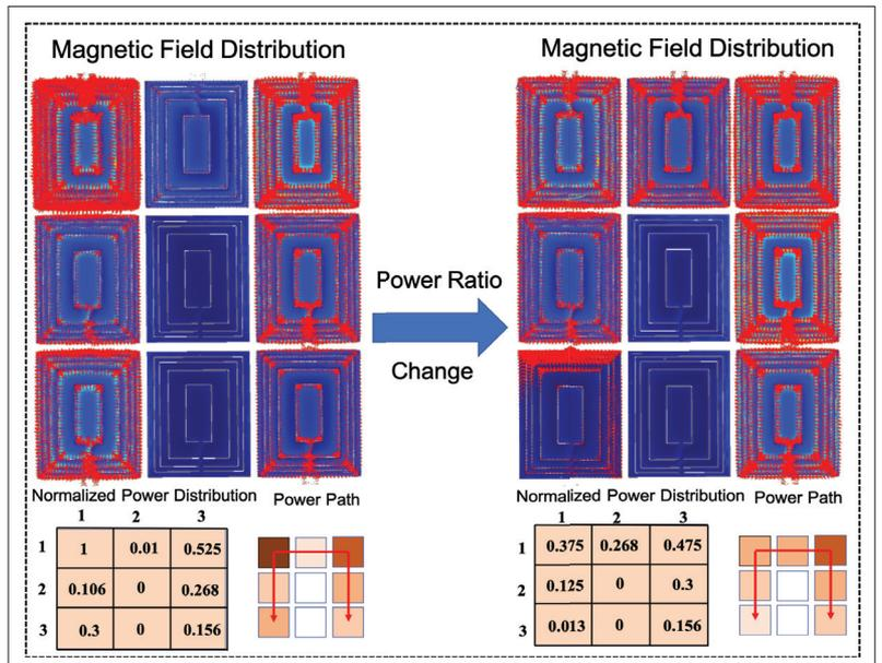
FIGURE 4. Simulation of power distribution of 2D surface for two different RIS configurations.
