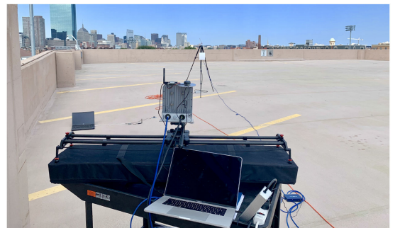
Fig. 15. Initial tests with sounder Tx mounted on slider.
